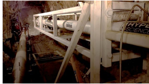
HyperSciences integration of the first HyperBreaker full Test Kit for the upcoming Field Trials. Fueled by clean Hydrogen and/or Propane (Planned Future: biodiesel)
