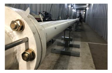
Our 100mm (4 inch diameter) system is currently being commissioned at the HyperLab Test Facility as shown in the image above. This is the common HyperCore system where the shorter system on the green mobile rig shown in top picture is intended for tunneling and mining demonstrations replacing drill and blast jumbo rigs (bottom right image: Sandvik) and the longer ram accelerator based system in the lab is for government and commercial aerospace demonstrations.
